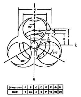
You must make sure that there is sufficient contrast for the symbol to be clearly defined, if the sign, tag, or label has a background color.
